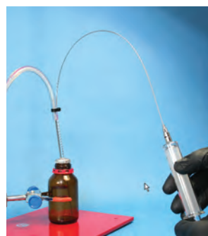
Fig. 8 Filling syringe using nitrogen pressure
