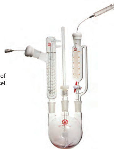
Fig. 9 Removing gas bubbles and returning excess reagent to the Sure/Seal bottle
