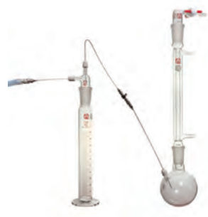
Fig. 13 Double-ended needle transfer with syringe valve
