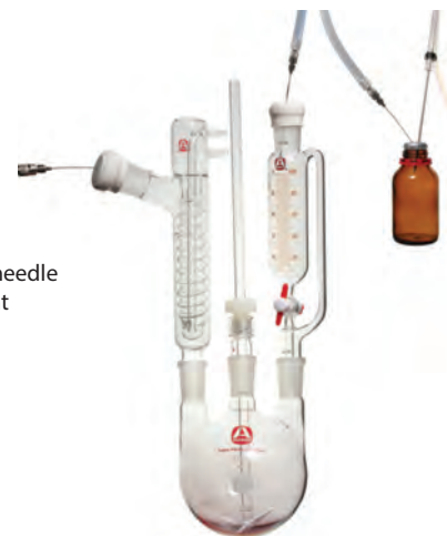
Fig. 13 Double-ended needle transfer with syringe valve
