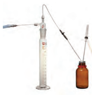
Fig. 12 Double-tipped needle transfer to graduated cylinder
