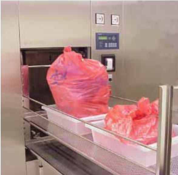
Biohazard bags placed in autoclavable secondary containers prior to autoclaving
